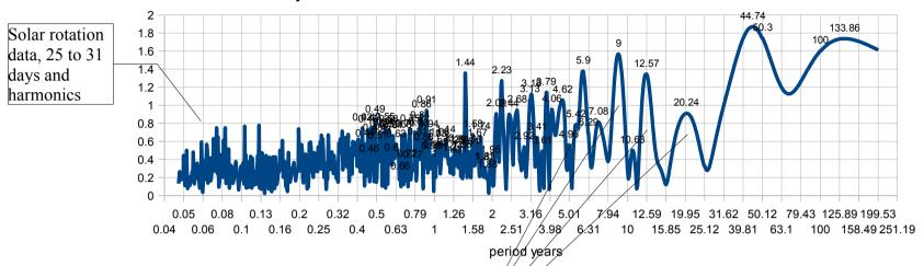
This shows an extreme spectrum range made practical by octave chirps. In practice this would not be normal usage. I've wiped some of the automatic data labels.
